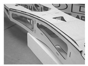
First sand the balsa formers flush with the sides and top of the fuselage and then you may round these formers off to give a smooth and flowing shape.
