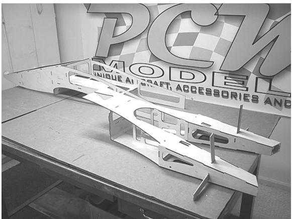
As you can see, the joining of the two sections is very straightforward. The bend in the back of the fuselage will require the use of masking tape as before to hold everything tightly in place while checking for squareness and fit.
