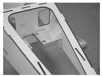
From the 1" x 1" x 36" balsa Triangle stock, cut four three inch sections and glue them above and below the forward gear mount as shown. NOTE: At this time you may want to go ahead and bolt the nose gear unit into place but it is not necessary. You can set up the nose steering servo without the nose gear in place.
