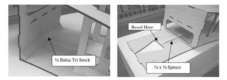
Check to make sure that all joints are securely glued and that the boom structure is straight and square. Some of the interior areas around the motor mount will be visible on the completed model. If you wish to paint or finish this area, now would be a good time. This concludes this portion of the assembly at this time.
