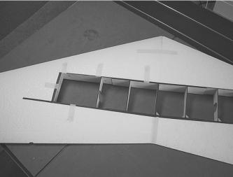
□ From the length of 1 x 1 balsa triangle stock, cut pieces to fit over the gear plate as shown to further reinforce this area.
