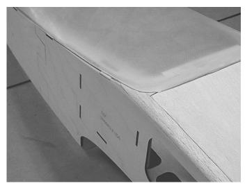
□ If you choose to, you may fill and sand the entire fuselage to your liking except for the underneath portion of the fuselage from the wing forward.
