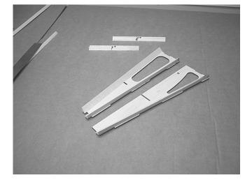
□ Use CA to glue the balsa triangle to the formers as shown and leave overhang at the rear. This will be sanded flush later.
