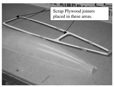
side. This is to keep from gluing the hatch to the model in the following steps.
